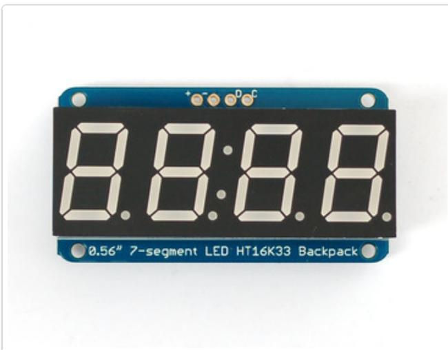
Remove the parts from packaging and place the LED matrix OVER the silkscreen side. **DO NOT PUT THE DISPLAY ON UPSIDE DOWN OR IT WONT WORK!!** Check the image below to make sure the 'decimal point' dots are on the bottom, matching the silkscreen.
