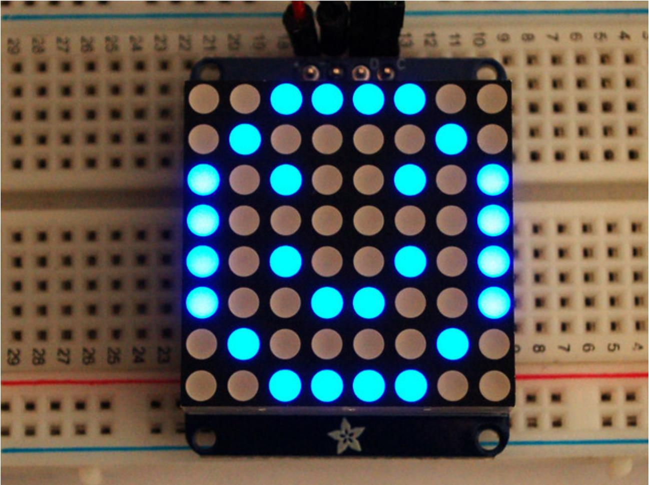
Once you're happy that the matrix works, you can write your own sketches. The 8x8 matrix supports everything the Adafruit GFX library - drawing pixels, lines, rectangles, circles, triangles, roundrects, and small bitmaps. [For more details check out the GFX page which will detail all of the GFX routines \(http://adafru.it/aPx\).](http://adafru.it/aPx)
