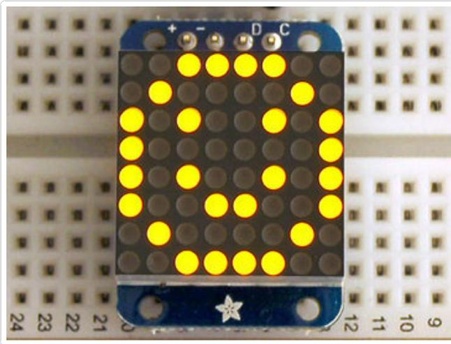
The default orientation for graphics commands on this display places pixel (0,0) at the top-left when the header is at the top and Adafruit logo at the bottom. `matrix.setRotation()` can be used to use the display in other orientations.
