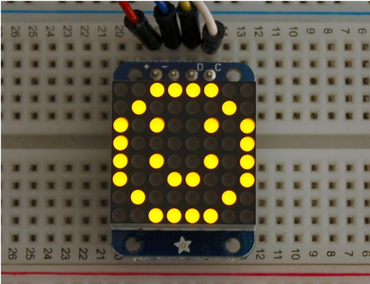
Once you're happy that the matrix works, you can write your own sketches. The 8x8 matrix supports everything the Adafruit GFX library - drawing pixels, lines, rectangles, circles, triangles, roundrects, and small bitmaps. [For more details check out the GFX page which will detail all of the GFX routines \(http://adafru.it/aPx\).](http://adafru.it/aPx)
