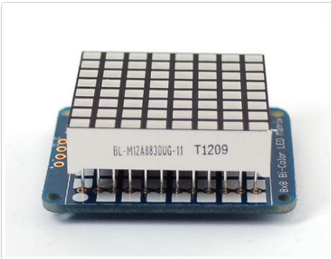
Remove the parts from packaging and place the LED matrix OVER the silkscreen side.
