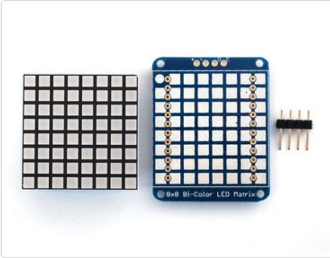
When you buy a pack from Adafruit, it comes with the fully tested and assembled backpack as well as a 8x8 matrix. You'll need to solder the matrix onto the backpack but its an easy task.
